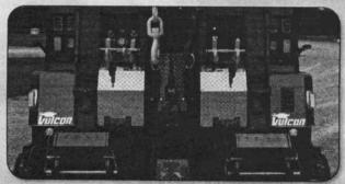
Rear tailboard provides quick access to lifting forks, air and electrical hook-ups, and safety chains, along with optional tailboard underlift controls.
